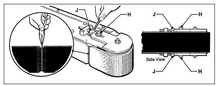
Figure 4-3 – Drive Belt Replacement/Tension Adjustment
